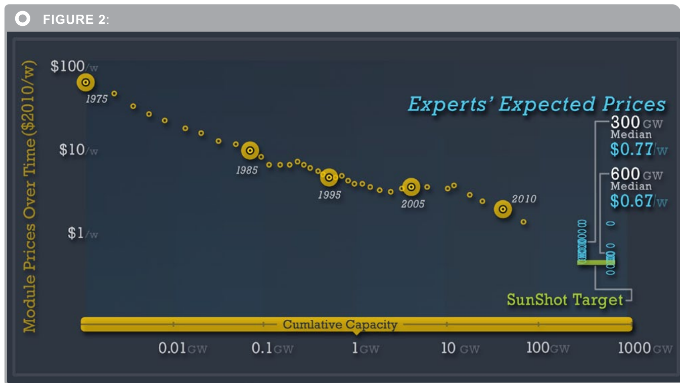
FIGURE 2: Falling prices for solar modules. As the total amount of solar modules produced has increased over the past few decades (from left to right), the price per watt has also fallen. Prices 1975-2009 are from Nemet (2009), and prices for 2010 and 2011 are based on data from Navigant and Bloomberg New Energy Finance. 5 Blue circles indicate the expectations from Near Zero's survey, for solar module prices at 300 GW and 600 GW of total installations (also called cumulative capacity). Also shown for reference in green is the module price target of the Department of Energy's SunShot Program.
